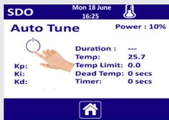
In PID mode, you can manually enter the P, I, and D value to optimise the control.
