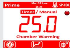
The run screen can be colour selected to suit the environment. The chamber will have default colours set depending on the model, but you can change colours to your preference. Both run screen text and background colours can be changed and as you change the colours, these are represented in the top bar.
