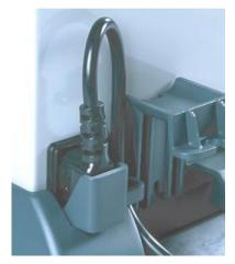
The carrier can be removed with a fingernail or tip of a screwdriver. A spare fuse is provided in the carrier.
