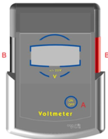
The d.c. meters will accept inputs of either polarity. If this polarity corresponds with the black (-) and red (+) input sockets, the display will simply show the figures. If the input polarity is reversed in relation to the input sockets, the figures will be preceded by a minus sign.
