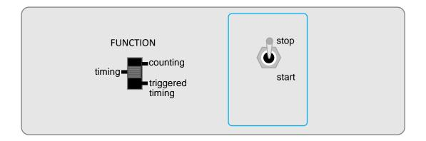
Timing is then **controlled by the stop/start switch**, and the instrument can be used this way for all experiments where a stopwatch or stopclock would normally be used. The display will count up in increments of 1 ms, to a maximum count of 999.999 s.
