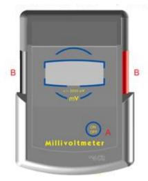
The d.c. meters will accept inputs of either polarity. If this polarity corresponds with the black (-) and red (+) input sockets, the display will simply show the figures. If the input polarity is reversed in relation to the input sockets, the figures will be preceded by a minus sign.
