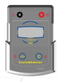
polarity. If this polarity corresponds with the black (-) and red (+) input sockets (C and D), the display will simply show the figures. If the input polarity is reversed in relation to the input sockets, the figures will be preceded by a minus sign.
