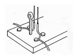
Finally, hold the armature level with the "eyes" of the split pins. Insert the knitting needle through one split pin, through the aluminium tube then through the second split pin, to make the axle of the motor.
