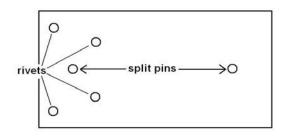
Do not push the rivets fully into the holes.
