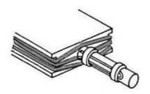
Finally, replace the rubber bands to hold the commutator in position. It is possible that one rubber band could hold the tips of the looped ends.
