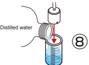
Procedure for repeated gas production (after step 14): Disconnect the small plugs from the tubes connected to the nozzles on the reversible fuel cell. This will allow water into the inner cylinders to replace the gasses and reset water levels to "0" line. Re-insert the plugs into the tubes and repeat electrolysis again.
