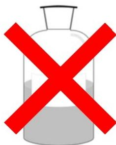
**DO NOT PUT ORGANIC SOLVENTS SUCH AS PROPANONE OR ETHANOL IN PLASTIC CUVETTES. USE TEST-TUBES OR GLASS CUVETTES FOR THESE.**
