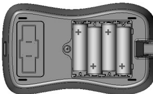
When the batteries need to be replaced the display will show *bAt* on startup.
