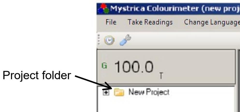
The left side of the screen displays, below the current readings and settings from the colorimeter, a list of the experiments and data sequences contained in the project folder, (double click the project folder and experiment files to view these).
