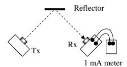
The path length should be ~1.5m. Switch Tx and Rx on (without horns). Turn Rx gain clockwise, then turn Tx tune until the meter reading goes high (usually off scale). In turn, decrease Rx gain and readjust Tx tune until a full-scale reading where Tx tune is at the maximum position.
