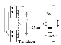
Connect the transducer to the monitor and earth terminals on the transmitter. The transducer will now emit a signal with the same amplitude and phase as the transmitter. (Twin or separate leads are satisfactory up to a separation of 1m). If a meter rule is secured on the bench, and Rx moved up and down it, minima and maxima are observed, the separation of which depends on x which represents to the distance between slits in a Young's optical experiment. Doppler Effect and "Beats"
