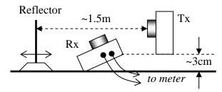
the distance you moved the reflector) is half the wavelength. The typical result is 4mm corresponding to a wavelength of 8mm.
