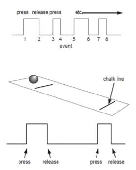
Suppose there was a start and finish chalk line on a bench and a ball bearing was rolling down the bench.
