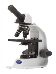
Monocular microscope, 400x, HC objectives
