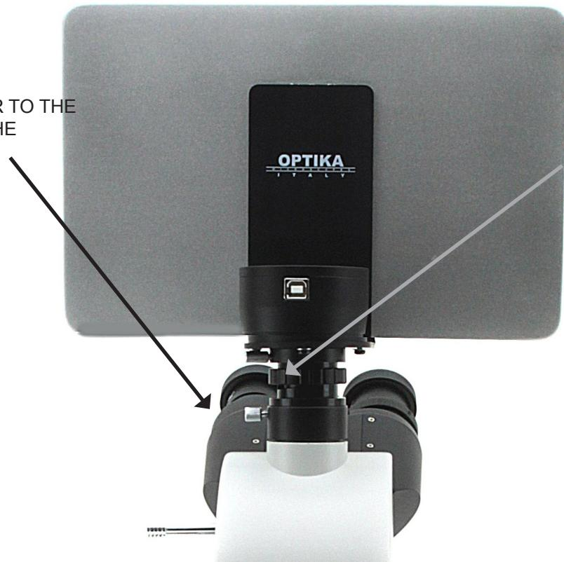
**2. PLACE THE MOUNTED ADAPTOR INTO THE PHOTO PORT AND LOCK THE SCREW**
