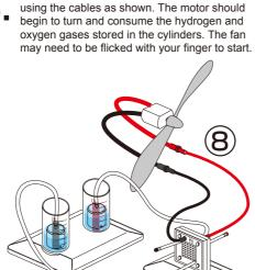
Connect the motor to the reversible fuel cell
