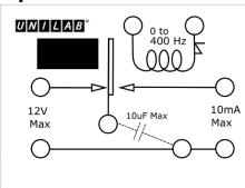
The Reed Relay must be driven by a signal generator capable of delivering a 5V square wave at a minimum current of 10mA. The reed switch module is extremely low capacitance and so will contribute a negligible error to any experiment.
