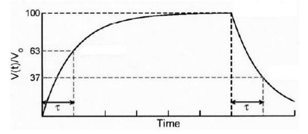
$\tau$  is known as the time constant and  $\tau$ =RC. A capacitor that is charging will reach 63% of its final value in one time constant. A capacitor that is discharging will reach 37% of its initial voltage in one time constant. A capacitor is fully charged (or discharged) after five time constants which is another way to measure the capacitance.
