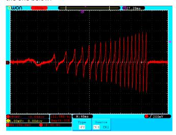
It is apparent that the time between adjacent peaks becomes smaller as the magnet accelerates down the tube. Decreasing the time base allows us to zoom in so that more accurate measurements can be made. Use the oscilloscope cursors to measure the time between successive peaks, then use the horizontal position control to move the next two peaks into view and repeat the process until the time between all the peaks has been recorded. Change the time-base as necessary to achieve the best results.
