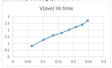
Draw a line of best fit and calculate the gradient to give an approximation for the acceleration due to gravity.
