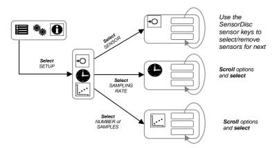
To start recording sensors - leave the menu and press the *Select* key. To stop recording, press and hold the *Select* key.
