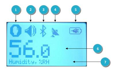
① Run/Stop icon – shows when the SensorDisc is logging data, or when the SensorDisc is not logging sensor data.
