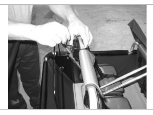
3) When you tighten the screw in the tapped bushing you hold the nylon fitting and the bushing fixed with your left/right hand as shown on picture #3. To tighten the screw you have to turn clockwise.
