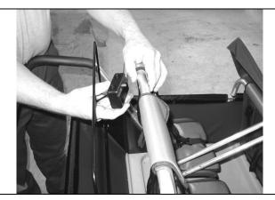
2) Place the screw from the plastic bag in the mounting hole of the nylon fitting and place the nylon fitting on the tube; remember to have the milled groove up so the hole for the locking spring is to the right as shown on picture #2.
