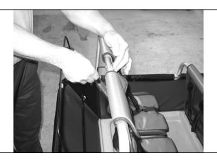
1) Remove the screw from the tapped bushing; hold a finger on the head of the bushing as shown on picture #1. To loosen the screw you have to turn <u>counterclockwise</u>.
