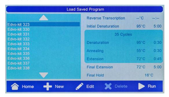
Selecting a protocol on the Load Saved Program screen will display information on the times and temperatures for each step. Disabled steps will be indicated by dashes in the temperature and time values. Tapping on the up and down arrows will allow you to scroll through additional programs.
