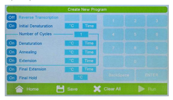
The Create New Program page allows you to edit, save, and run a new program. **NOTE: The "Run" button will not be selectable until a program has been saved.**
