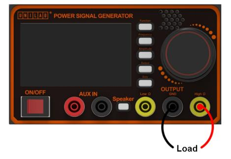
• Outputs displayed in gray indicates disable waveform output. Please make the connections as shown in the diagram below.
