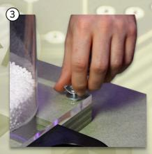
Place a washer, followed by a wing nut, onto each stud and tighten down.
