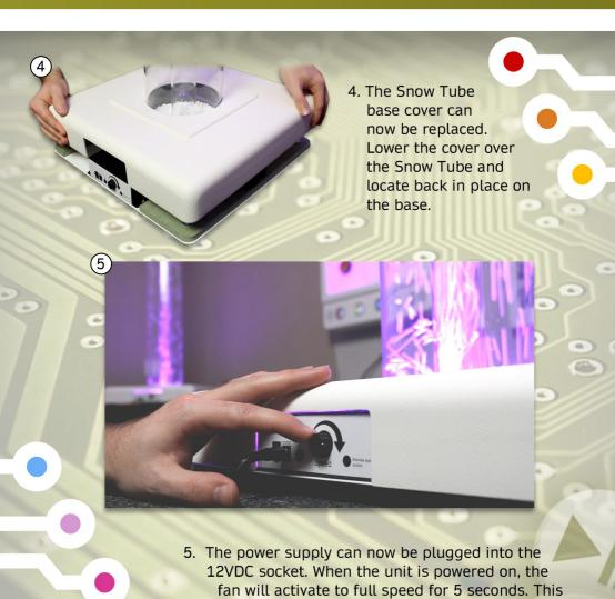
is to dislodge any of the snow particles that may have become stuck. Once the fan has finished this startup sequence, the dial can be used to set the desired fan
